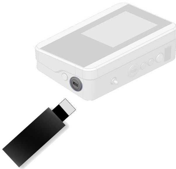
*Figure 29: Connecting the USB stick to the IC-Flow Controller*
